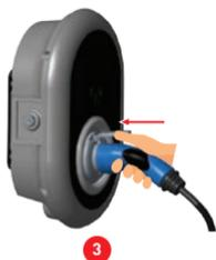
6- Turn on the power to your charging station. The cable becomes locked and the charging station starts behaving as an attached cable model.
